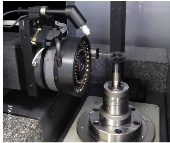
4 Measuring a skiving wheel on a Werth VideoCheck VHA; measurement and evaluation software: HAWK
